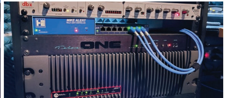
PHOTOS CLOCKWISE FROM LEFT: DEE DOTSON - LAKESHORE PUBLIC MEDIA'S REGIONALLY SPEAKING CO-HOST AND PRODUCER IN THE STUDIO / NEW TELOS AXIA RADIUS BROADCAST CONSOLE / INTEGRATED CONSOLE ENGINE WITH DSP-BASED MIXING.
